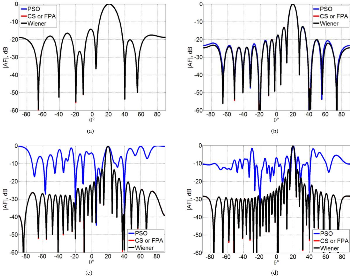
**Figure 3.** Optimal radiation patterns for SOI at  $20^\circ$  and two SNOIs at  $-20^\circ$  and  $40^\circ$ .  $M$  equals (a) 8, (b) 16, (c) 24, and (d) 32 elements.
