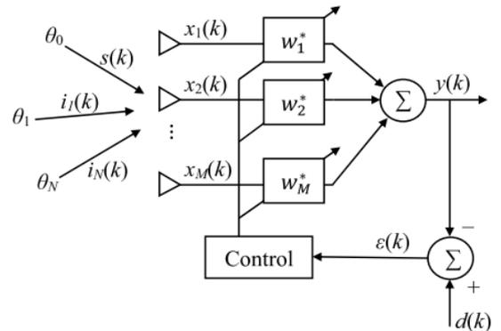
Figure 2. Adaptive beamformer for phased array antenna system.
